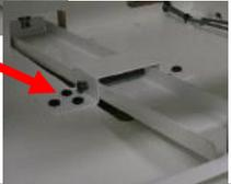
Move forward if latch does not lock door. Move backward if door has play when locked.</p> <p>Faulty wires. Check connections from solenoid to Controller Board. (AACE15514)</p> <p>If 12 Volts DC is at solenoid: Replace solenoid. (A5SO5052)</p> <p>If no 12 Volts DC at solenoid: Replace cables and/or controller board. (AACE15514, AACB15502)</p> |
