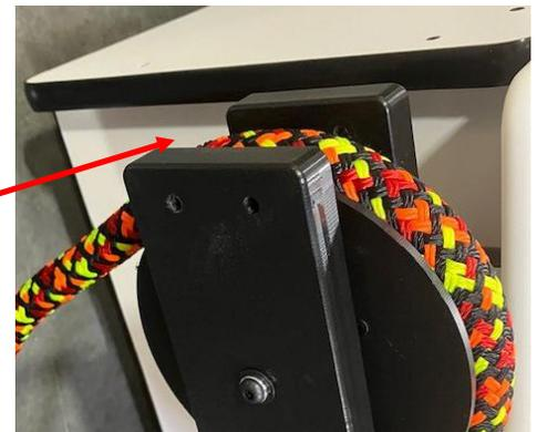
Bring the rope to the front of the cabinet and slide around the front pulley into the front pulley slot.
