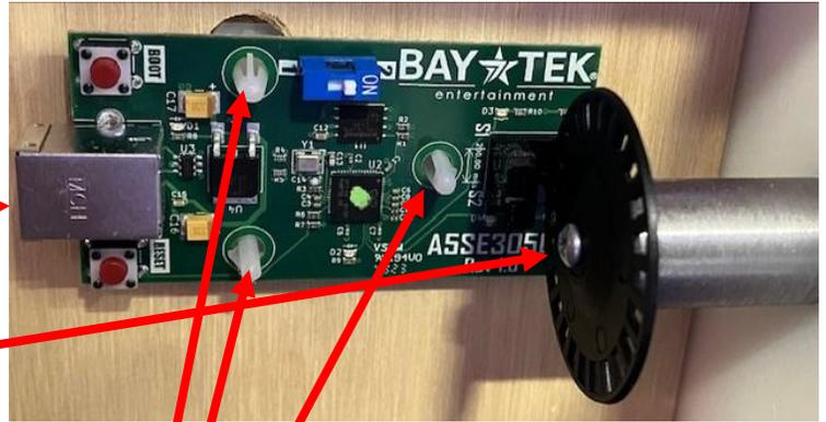
Unscrew the Encoder Wheel using a Phillips screwdriver. Remove the Encoder Wheel and set aside for later installation.
