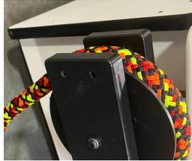
Replace the 2 bolts using a Phillips Screwdriver.
