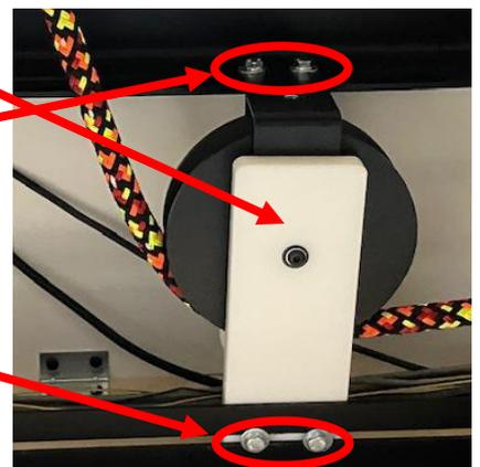
Re-install the Front and Rear Rope Channel White Plastic Covers by installing the 10 Phillips bolts with a Phillips screwdriver.
