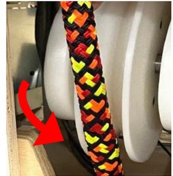
The rope should now be positioned so there is some slack at the lower rear pulley.
