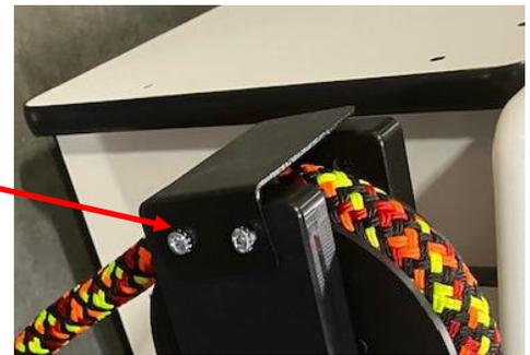
The rope should now be positioned so there is some slack at the lower rear pulley.
