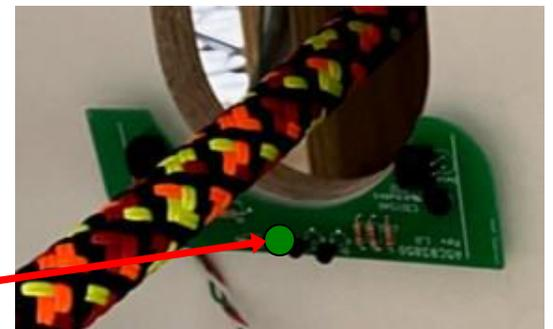
Rope Sag Sensors have 12 VDC between the red and green wires.
