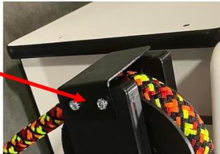
Bring the rope to the front of the cabinet and slide around the front pulley into the front pulley slot.
