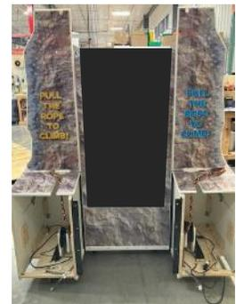
Using 2 people, carefully tip the main rear cabinet onto its back so the top monitor can be attached.
