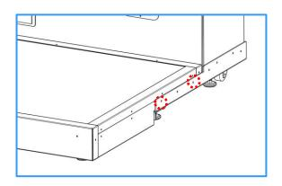
3) Install the floor LED cover with white 10-24 x 1¼ screws.
