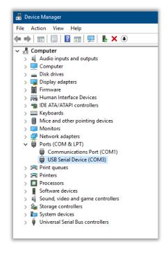
Verify that the "USB Serial Device" is set between COM2 to COM9.
