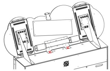
8) Secure the center header with black 10-24 machine screws.
