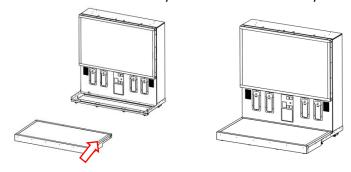
2) Secure the floor assembly with the provided white  $10-24 \times 1\%$  screws Repeat for the other side
