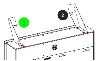
6) Position the 2 side headers by installing M4 screws between the brackets and the monitors
